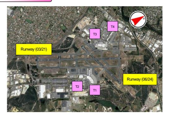
Flights are serviced by two runways; the main (03/21) runway, 3,444m × 45m and cross wind runway (06/24),  $2,163m \times 45m$ .
