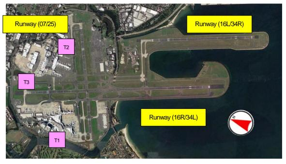
There are three runways at SYD. The main runway is (16R/34L) running north and south with 3,962m and the parallel runway of (16L/34R) with 2,438m. The cross wind runway of (07/25) is running east and west with 2,530m.
